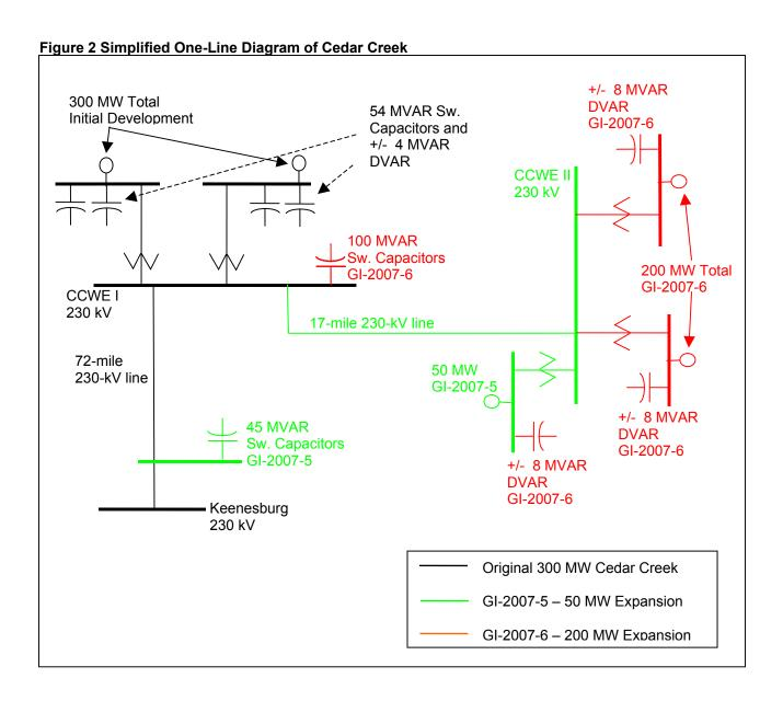
Based upon documentation provided for the Clipper C-93 wind turbines, these units do not attempt to regulate voltage or frequency and thus should be modeled in the power flow analyses as simple generators with a fixed reactive power capability. For this study, a 0.995 power factor was assumed, such that generator reactive power output
